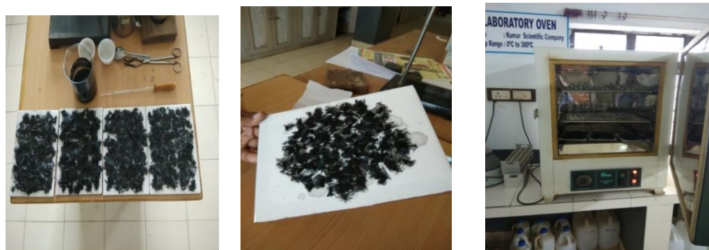
Fig 2.5 Grafting MWCNT-F on CF Surface
